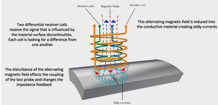
The eddy currents move on the surface of the conductive material because of a higher excitation frequency. Surface condition and the presence of surface defects has an effect on the magnetic field
